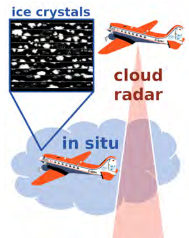
Fig. 7: Schematic measurement strategy to obtain quantitative measures of riming by comparing simultaneous cloud radar and in situ ice crystal observations.
