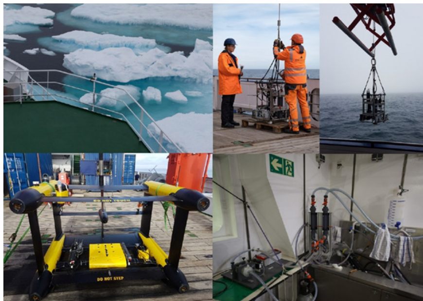
Fig. 4: Optical instrumentation used during MSM93 to hyperspectrally measure the absorption, attenuation and radiation of underwater light with active and passive instrumentation: At the discrete stations with the optical package (upper two right panels), towed behind the ship mounted on the Triaxus (lower left panel) and permanently during the entire expedition with an instrument operated with surface water pumped via a flow-through setup in the ship's laboratory (lower right figure). Photos from Julia Oelker IUP & AWI, and Tim Kalvelage.
