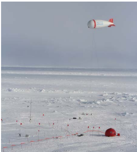
Fig. 7: Left: The meteorological measurement site including several turbulence and radiation instruments at the ice camp. Above everything floats the tethered balloon. The balloon group anxiously monitors the position of the balloon, which is attached to a winch (Photos: Marlen Brückner). Right: The two (AC) 3 A02 PhD students Matthias and Ulrike with their working tool. Thomas tries to free the balloon rope and the broadband radiation sonde from ice (Photos: Matthias Gottschalk).
