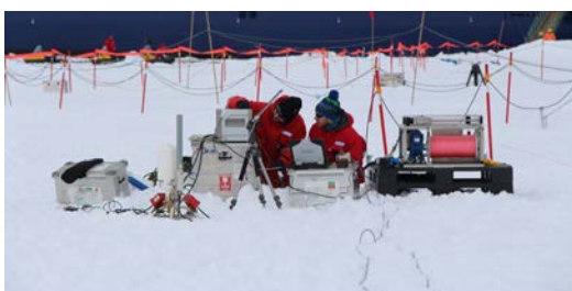
Fig. 7: Left: The meteorological measurement site including several turbulence and radiation instruments at the ice camp. Above everything floats the tethered balloon. The balloon group anxiously monitors the position of the balloon, which is attached to a winch (Photos: Marlen Brückner). Right: The two (AC) 3 A02 PhD students Matthias and Ulrike with their working tool. Thomas tries to free the balloon rope and the broadband radiation sonde from ice (Photos: Matthias Gottschalk).
