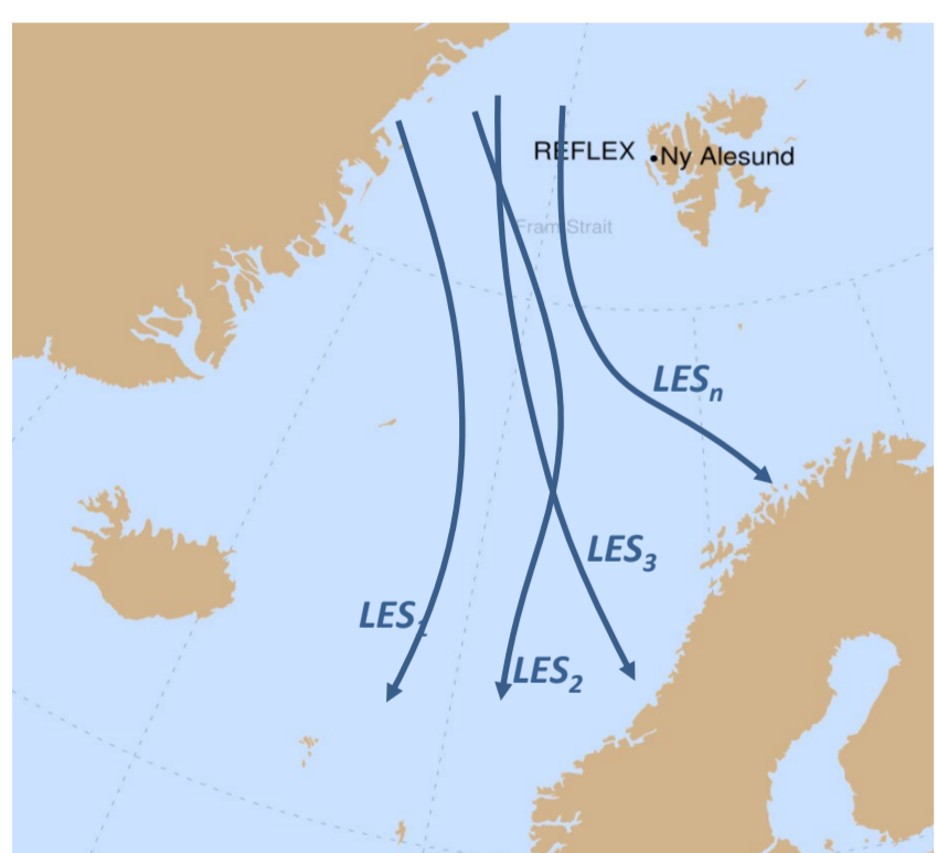
Fig. 3: Schematic illustration of an ensemble of Lagrangian LES realizations (driven by ECMWF analyses) along CAO-trajectories through the Fram Strait
