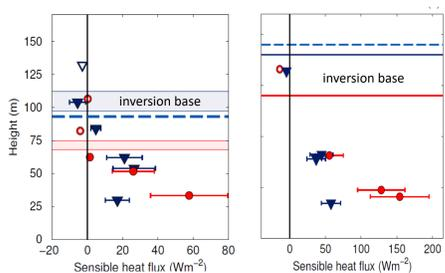
Fig. 3: Examples of aircraft measured linear and nonlinear flux profiles in the vicinity of leads (Tetzlaff et al. 2015, QJRMS).
