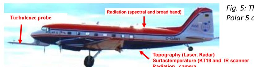
Fig. 5: The aircraft Polar 5 of AWI
