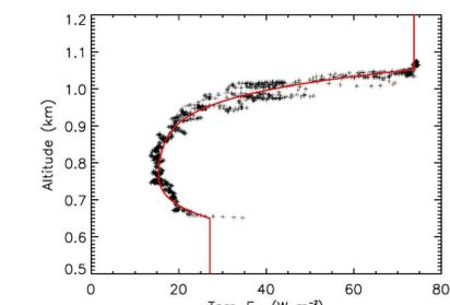
Fig. 4: Examples of aircraft measured net irradiances collected during the VERDI campaign using Polar 5.
